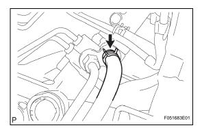
(c) Disengage the clip and disconnect the return hose.
