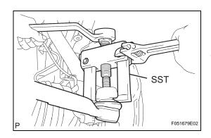
(b) Using SST, separate the tie rod end from the steering knuckle arm.
