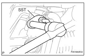
(b) Using SST, loosen the flare nut and separate the pressure feed tube.
