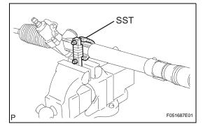
(b) Using SST, fix the steering link between aluminum plates in a vise, as shown in the illustration.
